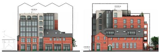
Figure 14 - Proposed scale and massing, with the comparative dismissed at appeal scheme outlined - <u>please note that the proposed materials shown differ to those now proposed</u>)
