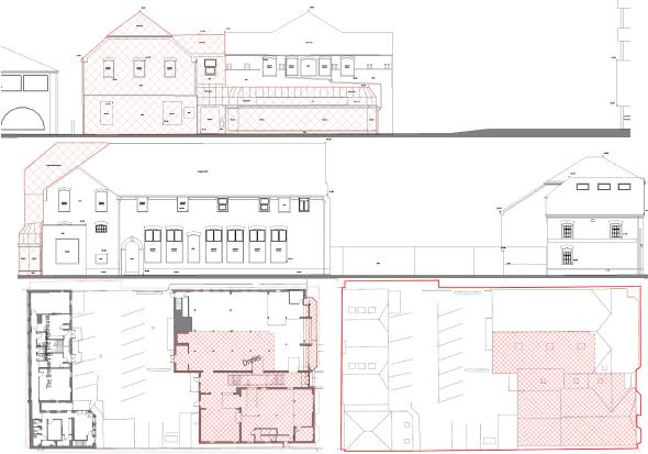
Figure 12 - Extent of proposed demolition hatched
