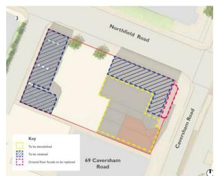
Figure 4 - The extent of retention and demolition of existing site buildings
