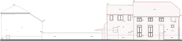
South elevation - demolition shown in red
